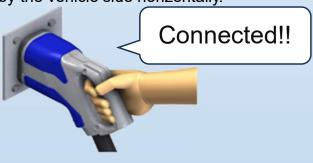
2. Pull the connector straight from the inlet by the vehicle side horizontally.
