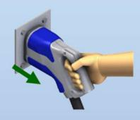
2. Insert the connector straight into the inlet by the vehicle side horizontally.
